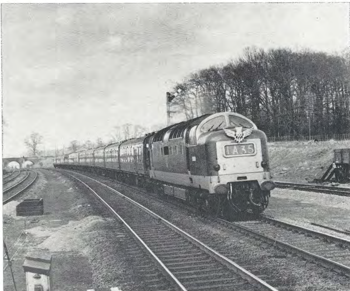
The "Flying Scotsman", non-stop over the 268½ miles from Newcastle to King's Cross in 233 minutes, hauled by 3,300 h.p. "Deltic" diesel No. D9010 The King's Own Scottish Borderer , with its handsome thistle headboard, passing St. Neots. [Eric Treacy
