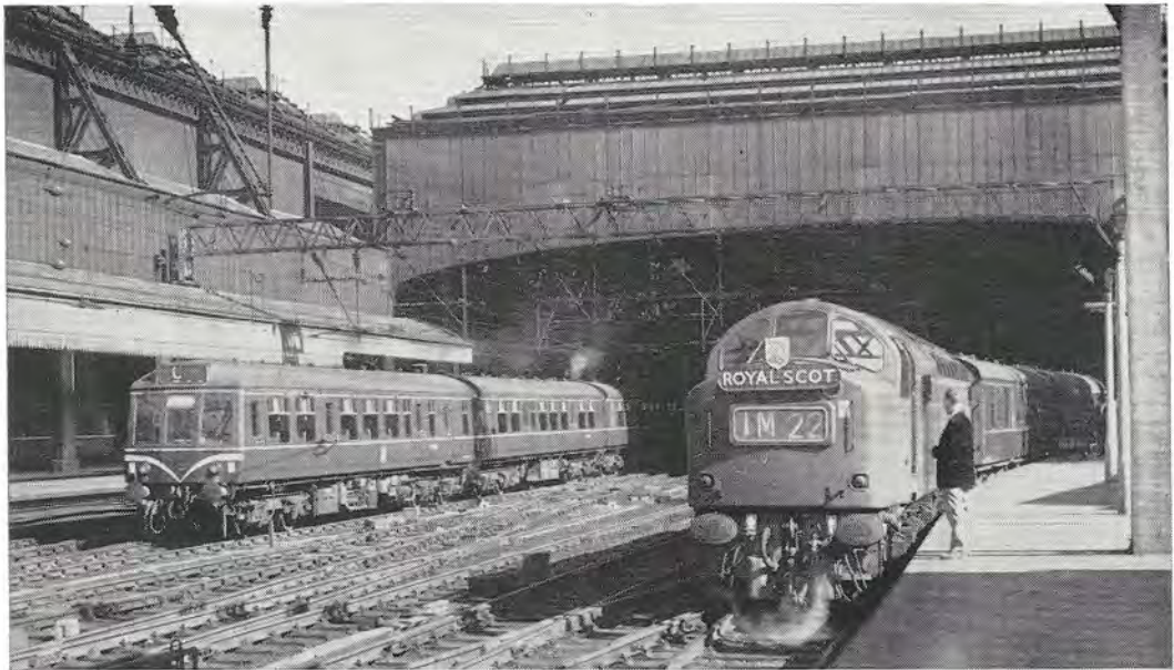
★ A Derby-built three-car diesel multiple-unit leaves Glasgow Central, passing an English Electric Type '4' diesel on the south-bound 'Royal Scot'. [B. Haresnape]
