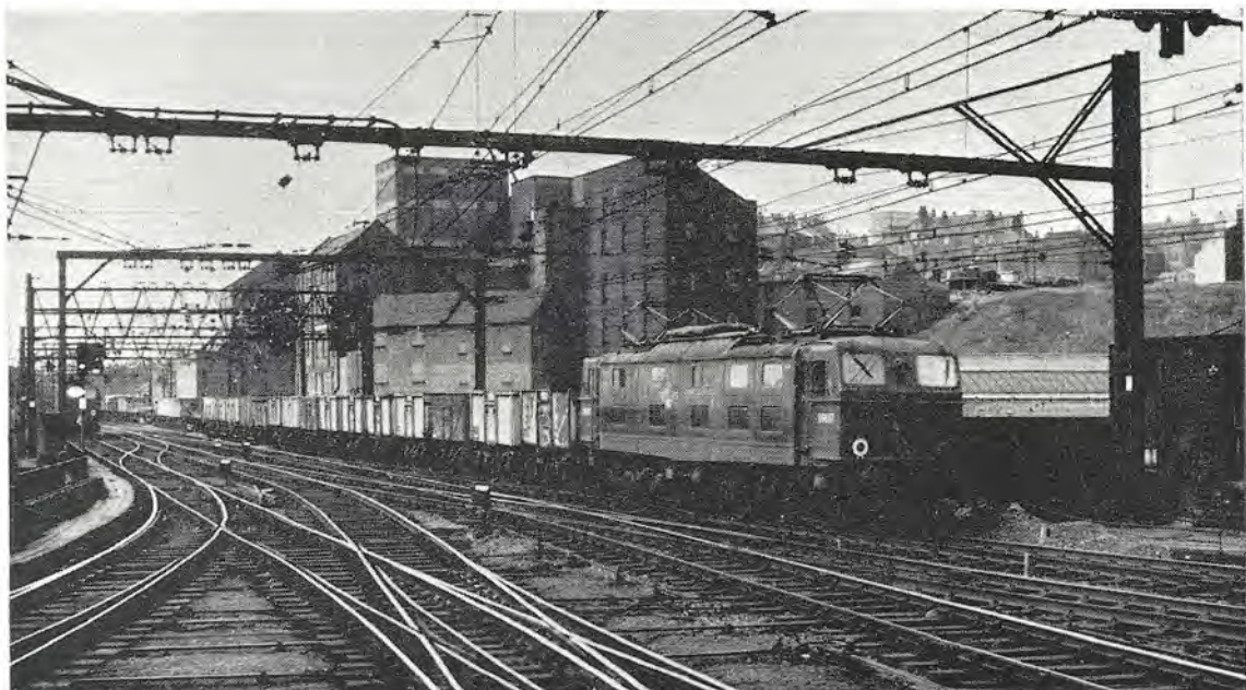
Britain's first all-electric main line. The Manchester-Sheffield line electrification was completed in 1954 on the 1,500 volts d.c. overhead system. Class EMI Bo-Bo No. 26037 approaches Sheffield Victoria with a haul of coal empties.
